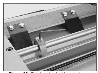
Figure 22. Chip breaker height adjustment.
